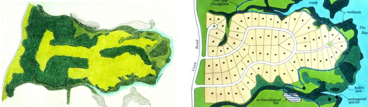
Figures 19-5 A and B: Predevelopment Situation and "Yield Plan". The land prior to development, shown in Fig. 19-5A, consists of roughly 80 percent upland, almost equally divided between farmland and forest, with the remainder being wetlands and floodplains. The conventional layout of 72 houselots (Fig. 19-5B) also serves as a "Yield Plan", demonstrating the number of houselots the property would ordinarily support in a standard plat with no usable open space. Source: Arendt 1993
