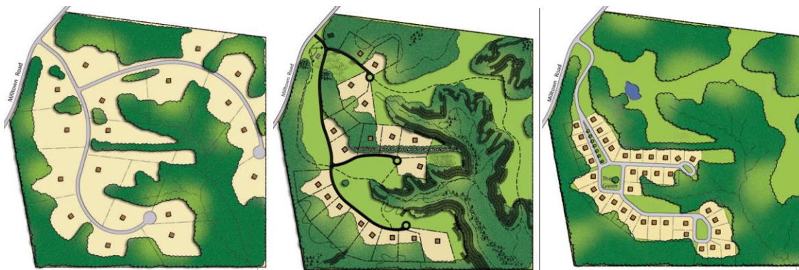
Figure 19-15: Eighteen lots are shown on the conventional "Yield Plan" on the left (at a two-acre size) and on the conservation design in the center with one-acre lots, where half of the buildable land has been preserved as permanent open space (in addition to the unbuildable soils and slopes). Double density is shown on the right, with 36 quarter-acre hamlet lots, where 70 percent of the buildable land has been conserved. Density increases generally obligate applicants to provide special benefits to the community, such as significant increases in open space, land dedication to the municipality or land trusts, and/or affordable housing. Source: Arendt 1999 and Natural Lands Trust
