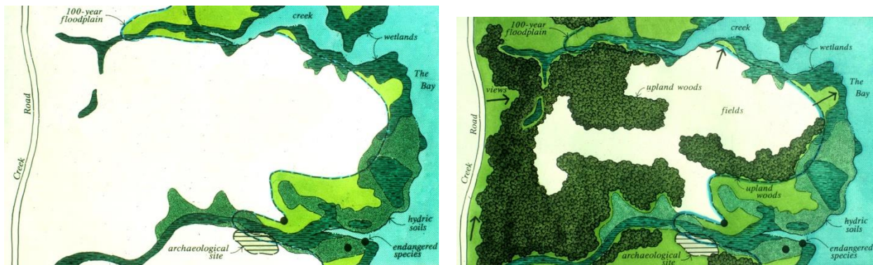
Figures 19-6 A and B: Step One, Identifying Primary and Secondary Conservation Areas. The first step involves identifying Primary Conservation Areas (Fig. 19-6A, limited to wetlands, floodplains and steep slopes), and Secondary Conservation Areas (Fig. 19-6B) including those unprotected elements of the natural and cultural landscape that deserve to be spared from clearing, grading, and development. In this example the mature upland forest habitat is of critical environmental importance, while the farmland's ecological value is negligible. Source: Arendt 1993
